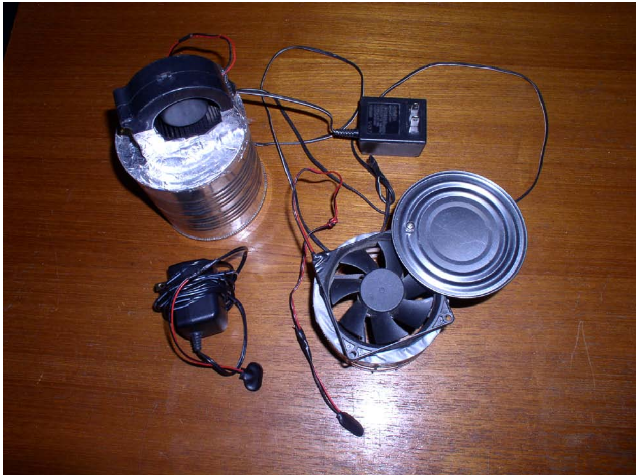
Figure 5 Typical small fan and blower, adapted for the J-RO
