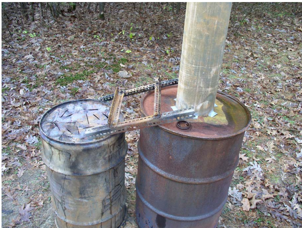
Figure 4 Modified Drums and support racks for the J-RO
